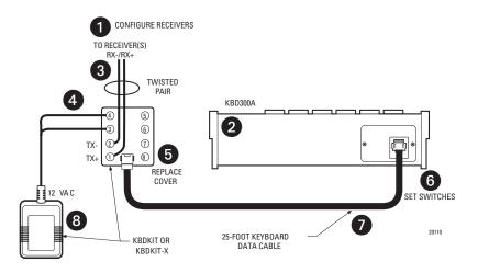
Figure 10. Direct Keyboard and Receiver Wiring
